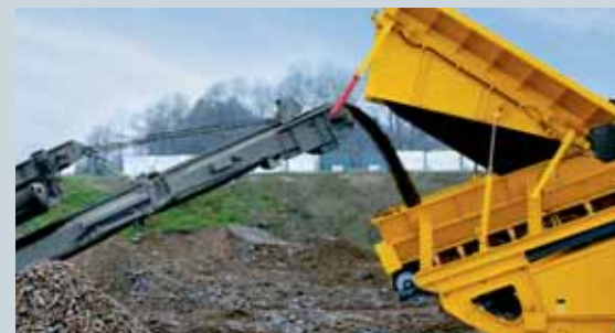
Besides a wheeled loader, a RUBBLE MASTER crusher can also be used for direct feeding.
