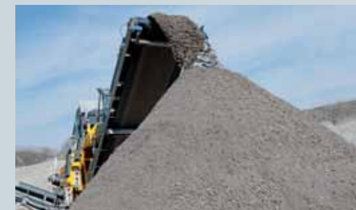
The long, hydraulic fold-in discharge belts can be adjusted steplessly up to 4 metres' discharge height.
